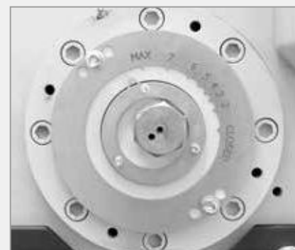
BB 500 XL: Continuous gap width adjustment
